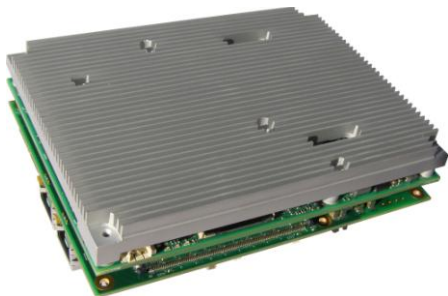
COM Express SBC Board Stack using the CB2600
